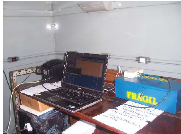
Figure 3 - Compact system for the detection of gamma rays. The scintillator and photomultiplier are inside the blue metal box.
